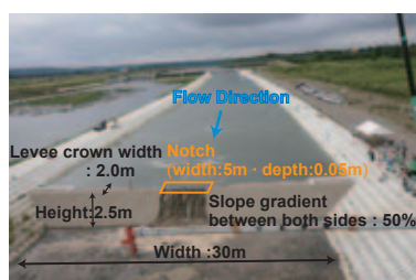
Technical evaluation using full-scale experiment
