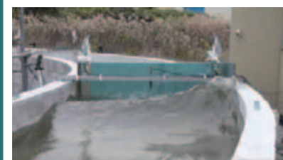
Understanding the effect on structures by experiment of tsunami running up a river
