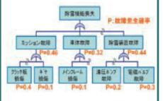
Analysis of probable failure of snow remóval máchines using FTA
