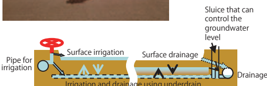
Mechanism of groundwater level control system
