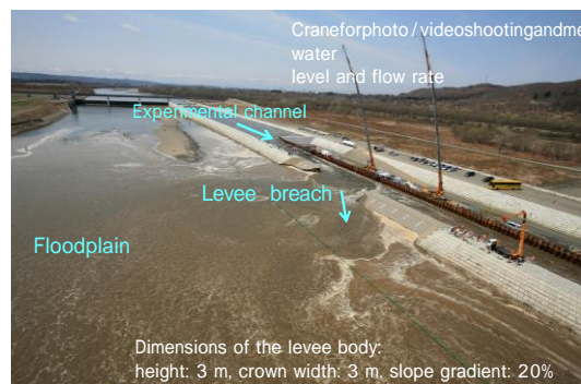
Figure 2. Experiment on a levee breach from overtopping
